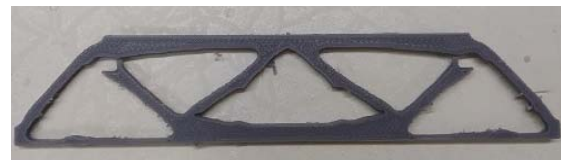
Figure 8: Topology optimized simply supported beam fabricated using FDM printer
